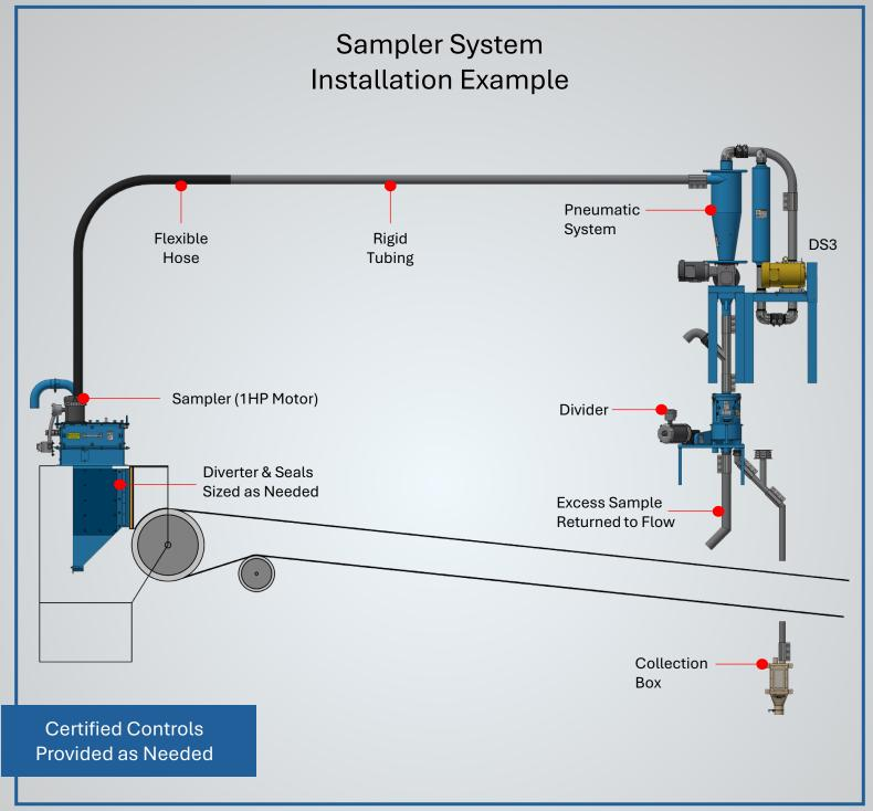
The Gamet 6400 Sampling System is intended for applications that require official sampling grades. This system is specifically designed to mount at the end of a belt, drag, or screw conveyor and is ideal for use in barge, ship, and rail loading applications. The sampler is used in conjunction with a pneumatic conveying system that extracts the sample from the diverter. Gravity applications can also be provided if necessary or space is a concern.
